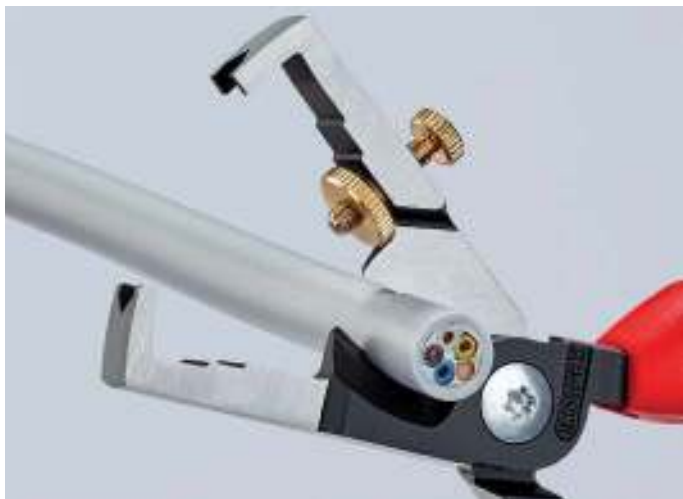
Induction-hardened shear blade with precisely ground cutting edges for crush-free cutting of copper and aluminium cables of up to Ø 15 mm (5 x 2.5 mm²)
