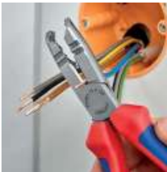
Cutting when shortening single conductors
